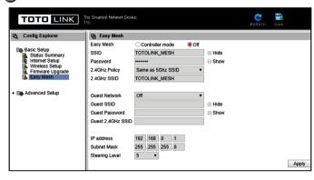
Firstly, select Controller Mode to enable Easy Mesh function. Second, set the SSID and Password of the Master Touter. Third, click APPLY. Then the router will restart after you click **YES** in the prompt box that appears. Please wait for the router to restart.
