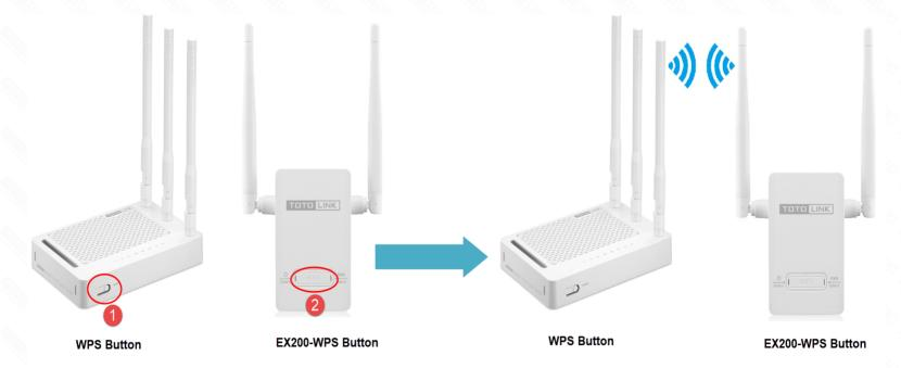
**Note:** The "extending" LED will flash when connecting and become solid light when connection is successful. If the "extending" LED is off lastly, it means that the WPS connection is fail.
