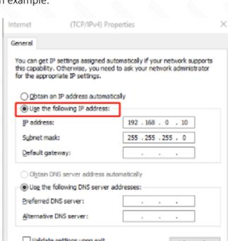
1-6. When you don't need to set the IP address manually, Please select **Obtain an IP address automatically** and **Obtain DNS Server address automatically**.
