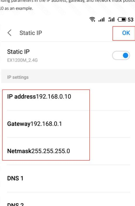
1-3. When you don't need to set the IP address manually, Please turn off **static IP**.
