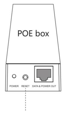
**RESET on PoE box** Press the RESET button on PoE box for about 8 seconds until the signal strength indicators blink.
